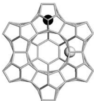
Figure 8. A [001] view of Ti-YNu indicating favorable substitution at the “rim” site (white) and less favorable incorporation at the “spiro” site (black).
